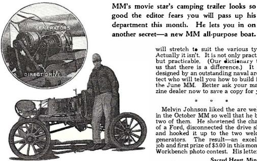
Melvin Johnson built two MM welding generators and mounted them on a shortened Ford. He wan first prize of \$5.00. Upper circle shows the two generators. Photo shows Johnson and welding outfit.
