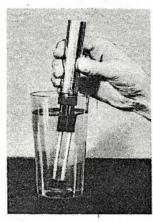
Batteries in handle of sterilizer send current between two silver electrodes immersed in the water.
