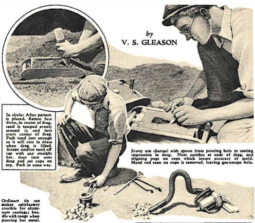
BRASS, bronze, or aluminum castings for model projects or even larger work can be made in your own "hole-in-the-ground" foundry at a cost of no more than one cent each--castings so accurate, so smooth that they are ready for use after only a few minutes on the buffing wheel.
