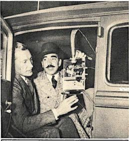
Left.—As experimental proof, Lear has mounted his device on an automobile. The loop aerial on the roof picks up the impulses, and the straight serial in the rear acts as a pointer, to make sure the plane will travel toward rather than away from guiding station. Above—The guiding set is shown installed in auto. It weights about 30 pounds and is equipped with a dynamotor which supplies power.
