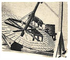
A dog, walking on this wheel, remains stationary; the geared wheel moves under him, making power to operate machinery.
