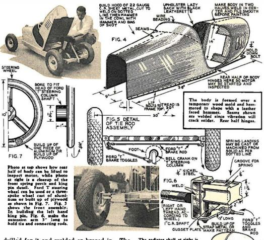
drilled for it and welded or brazed in. The wheels must be fitted with bronze bushings. Each wheel should be locked on with a double lock nut and the shaft threaded so that the nut tends to tighten in the direction of wheel rotation.
