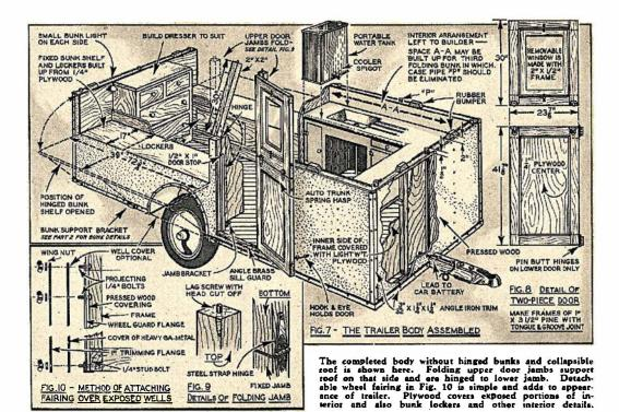
used. Sir Guy's trailer is rigged with Ford V-8 wheels but the bearers are long enough to take almost any standard spring assembly. This being so, select and fit your running gear taking care to align it correctly with the frame as the "roadability" of your trailer is intimately associated with this important item.
