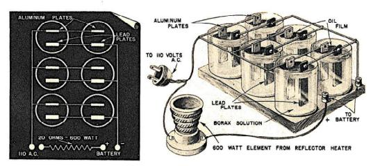
Construction of heavy duty electrolytic charger is shown above. Aluminum plates will gradually wear away, and may need replacement. Size of plates determines current which will pass; thickness determines life of plates. Pour film of clean oil over solution in each jar to prevent evaporation. Iron or copper may be used in place of lead. Baking soda (½ oz. to gallon of water) works as well as borax. Current density is about 100 ma. per sq. in. of immersed aluminum surface.
