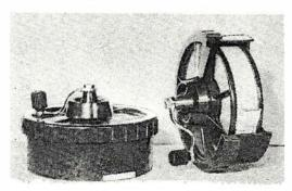
This unique developing tank can be carried aloft by aviators for processing serial films as quickly as they are taken. Lanks hold 25 feet of 35 mm. or 50 feet of 16 mm. film.
