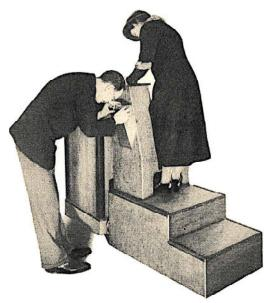
The customer puts foot through hole in machine and looks through the view plate to see how the shoe fits the foot.
