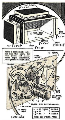
Mount parts on panel as shown. Make 2 mh. choke coil with 200 turns of No. 32 d.c.c. wire, jumbled, on pencil core.
