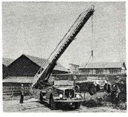
Fire ladder, used as a crane, rescues automobile after wreck.
