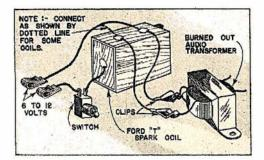
Spark Coil Repairs Burned Out Phones
