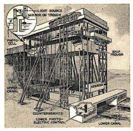
A ray of light, reflected by a mirror into a photo-cell, stops this huge water-filled elevator trough at the canal levels.
