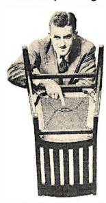
Four hooks are fastened to chair corners and tightened by awivel.
