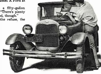
Tank of this Dieselized Model A Ford is filled with crenkcase drainings, not gasoline. In towing large car from Phoenix a Los Angeles, driver made 26 miles per gallon of fuel oil.
