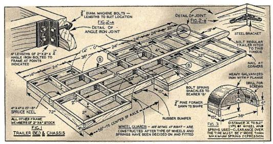
Complete details of the trailer foundation are shown above. Running gear available so the builder is attached to the bearers marked B. Flooring, laid diagonally over the frame, helps to strengthen it. Angle irons and brackets also brace it.
