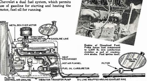
Drawing indicates thanges made by Don Redman in 1930 Chevrolet to permit use of either gasoline or fuel oil. Butire installation cast less than \$15. Jets of original carburetor are altered, and this used for fuel oil. New down draft carburetor is added as shown, to vaporise gasoline. Dual throttles and carburetors make the switch from gas to oil almost instantaneous.
