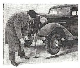
This "standup" jack permits the motorist to lift his car by the back bar of the humper, without even stooping or soiling his hands. A threaded shaft fits into the removable base and raises the car slowly but safely by crank-spinning.
