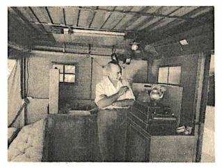
Here is the trim interior of Sir Guy Standing's trailer. On the sink at left is the portable water tank. Note folding table strapped to the roof. Pipes supporting roof and strengthening guy wires can be seen in rear.
