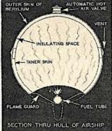
Hot air furnishes the lifting power for this newly-designed dirigible. Cross-section of hull (above) reveals inventor's unique method of using fuel for warming the inside stee of the giant bag.
