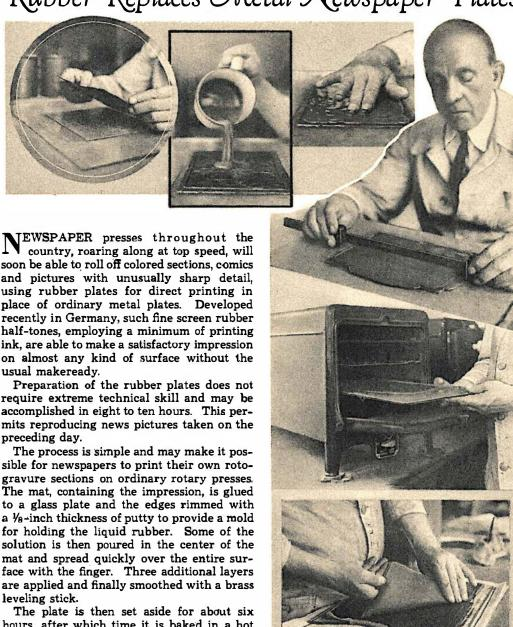
The plate is then set aside for about six hours, after which time it is baked in a hot oven. When the rubber has cooled, the plate is peeled from the mat and mounted on a wooden or metal base for flat-bed printing or backed with linen, cardboard or zinc, curved and clamped to the rotary press.
