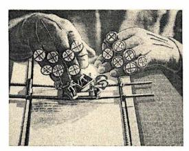
Radical in design, this "kid-glove" typewriter has its many character signs fastened to the fingers of the operator.
