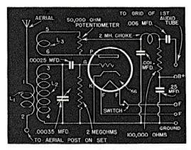
Potentiometer may be any value from 50,000 to 250,000 ohms. Rading for .25 mfd. condenser is 400 volts. Other condenser sizes are not critical—use closest size you have.
