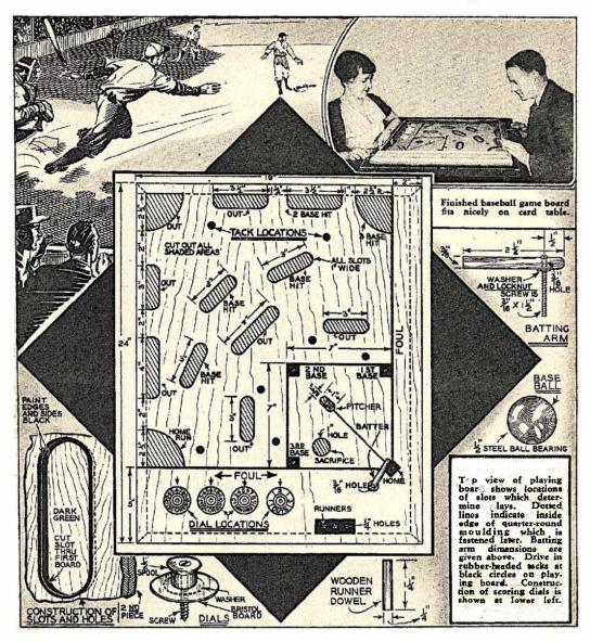
moulding to the blocks all around the board to form the sides. The plywood pieces are now fastened together with small screws around the edges. Nail a piece of wallboard to the blocks for a bottom covering.
