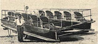
Left—Rear view of newly-built pontoon speed boat. Note the anti-wave-splash grooves which, dipping downward, tend to buoy up the stern. Right—Chairs for passengers are placed atop the framework into which the power unit nests.
