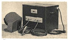
Electric arc welder operates without interruption. High frequency current maintains connection between electrode and work. Shield protects face from ultra-violet sunburn.
