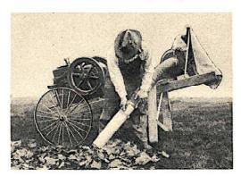
The gasoline motor, set on a two-wheeled truck, sets up a vacuum which draws the leaves up through suction pipe.
